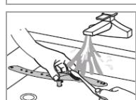
Check the outlet nozzles of the spray arm regularly for blockages.
