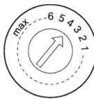
Take off the lid of the rinse aid dispenser and adjust the dial to the desired level. The factory setting is "4".
